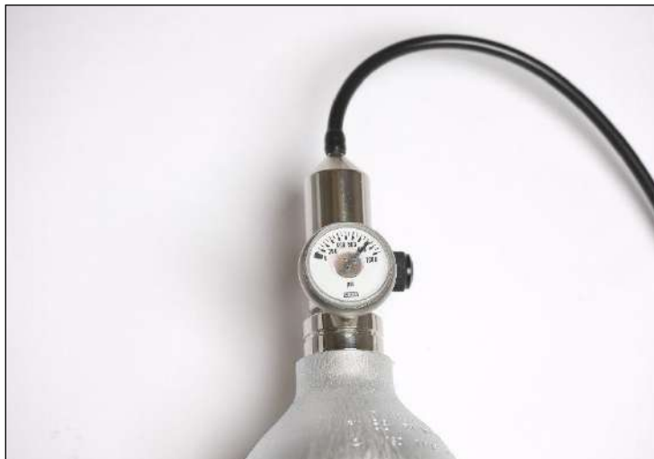
Figure 26 Flow Regulator Fitted to Calibration Bottle
