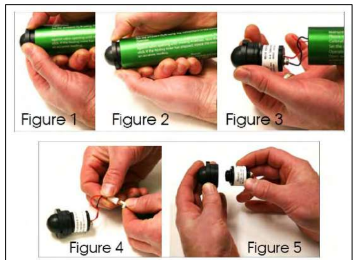
Figure 2. Removal and replacement steps.
