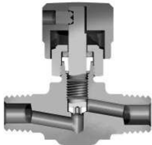
Figure 2: V4C Series Needle Valve Cross Sectional View
