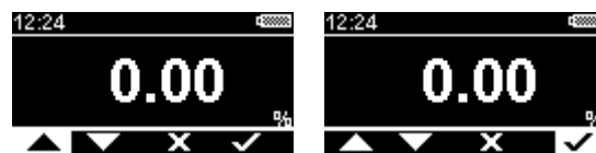
Figure 27 CO 2 LO calibration data entry screen (ready to confirm calibration)
