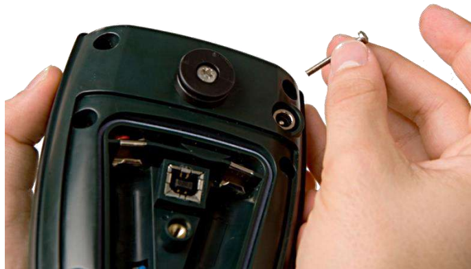
Figure 9 Replace the sensor cap and secure the screws
