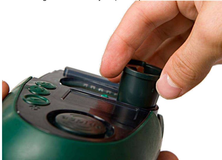
Figure 7 Remove the extraction tool
