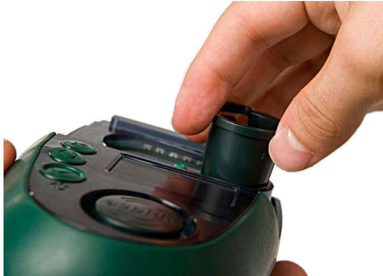
Figure 42 Remove the extraction tool
