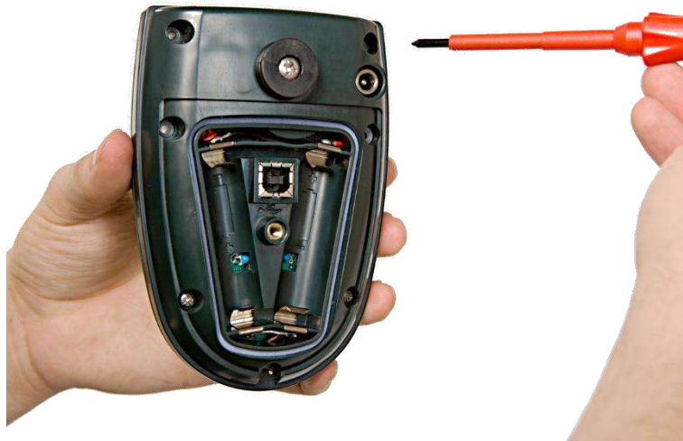
Figure 2 Remove the sensor cap screws
