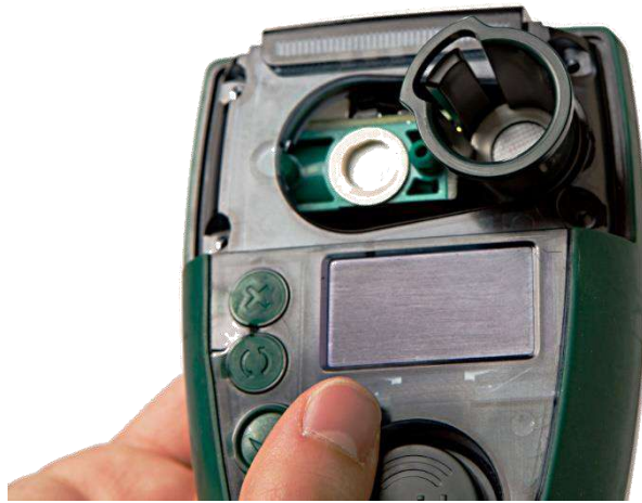
Figure 36 Correct extraction tool position
