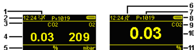
Figure 11 Dual sensor display (left), single sensor display (right)
