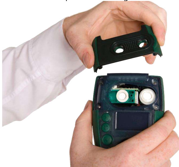
Figure 3 Remove the sensor cap
