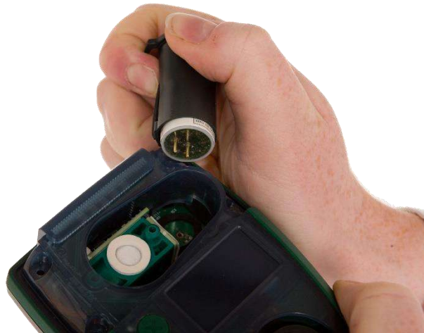
Figure 38 Removing the oxygen sensor
