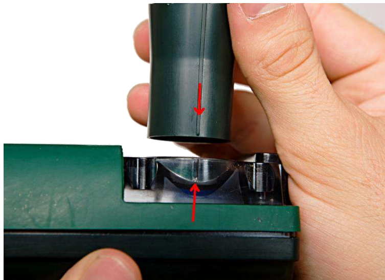
Figure 35 Align the extraction tool
