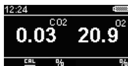
Figure 20 Carbon dioxide calibration due reminder
