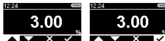
Figure 28 CO 2 HI calibration data entry screen (ready to confirm calibration)
