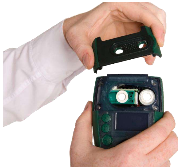
Figure 33 Remove the sensor cap
