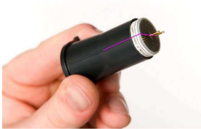
Figure 40 Align the new sensor in the extraction tool
