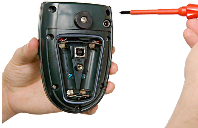
Figure 32 Remove the sensor cap screws
