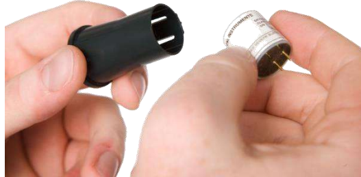
Figure 4 Insert the new sensor into the extraction tool
