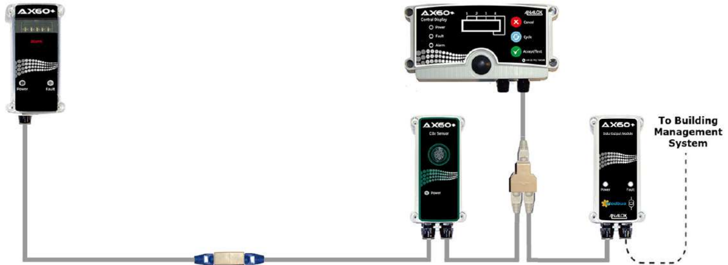
Example layout of quick connect system with data output module
