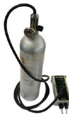
Step 4] Fit the regulator to the check gas bottle
