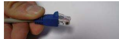
Slide boot back over lock clip
