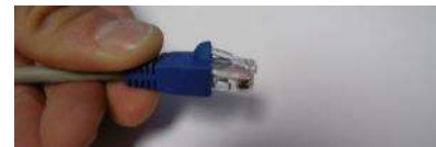
Slide boot back over lock clip
