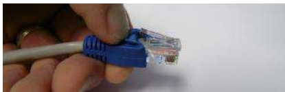
Pull boot back to access lock clip
