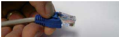
Pull boot back to access lock clip
