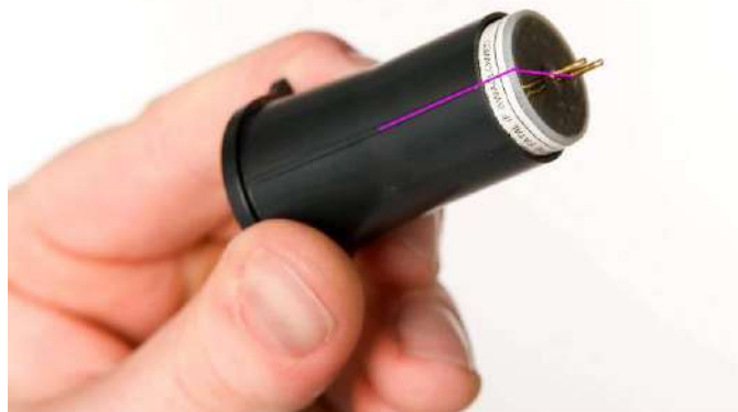
Figure 29 Align the new sensor in the extraction tool
