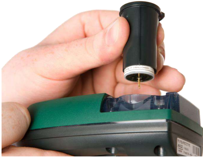
Figure 30 Align the new sensor with the Aspida device
