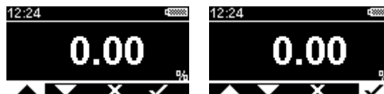
Figure 16 CO 2 LO calibration data entry screen (ready to confirm calibration)
