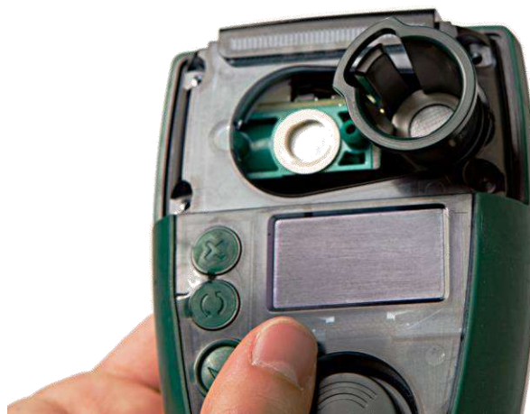
Figure 25 Correct extraction tool position
