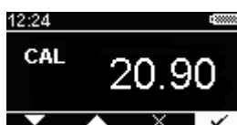
Figure 12 Calibration data entry screen (ready to confirm calibration)
