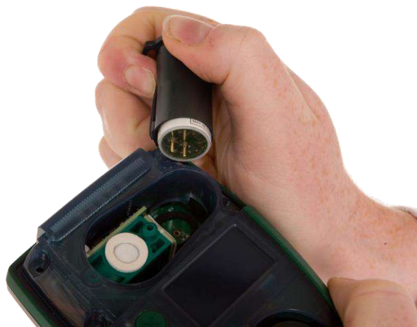
Figure 27 Removing the oxygen sensor
