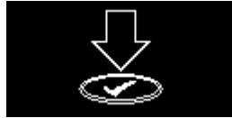
Figure 6 Display shown when the man-down alarm is triggered
