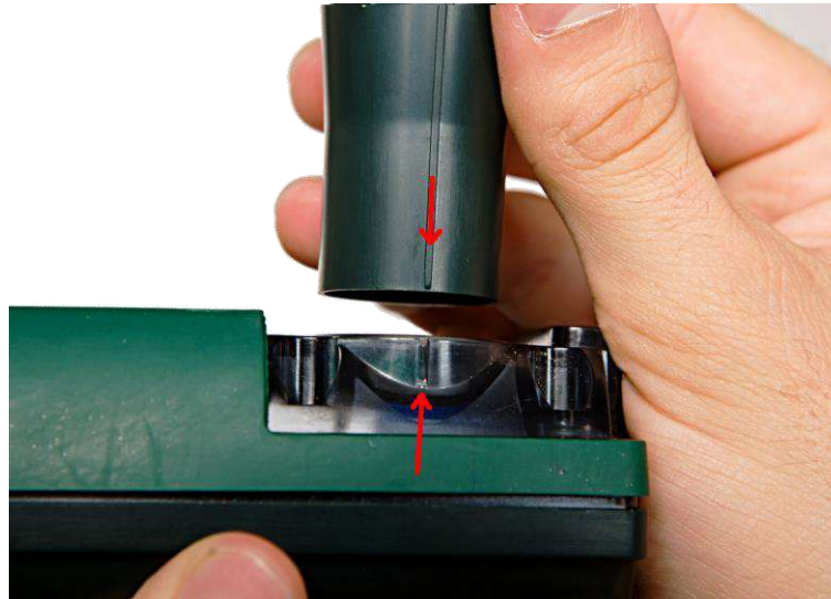
Figure 24 Align the extraction tool
