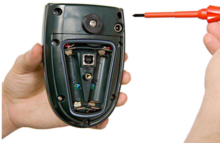
Figure 21 Remove the sensor cap screws
