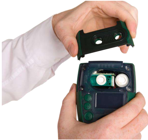
Figure 22 Remove the sensor cap
