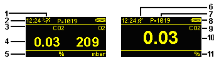
Figure 3 Dual sensor display (left), single sensor display (right)
