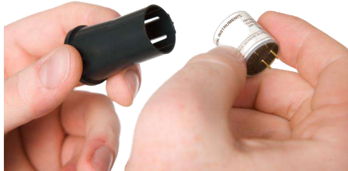
Figure 28 Insert the new sensor into the extraction tool
