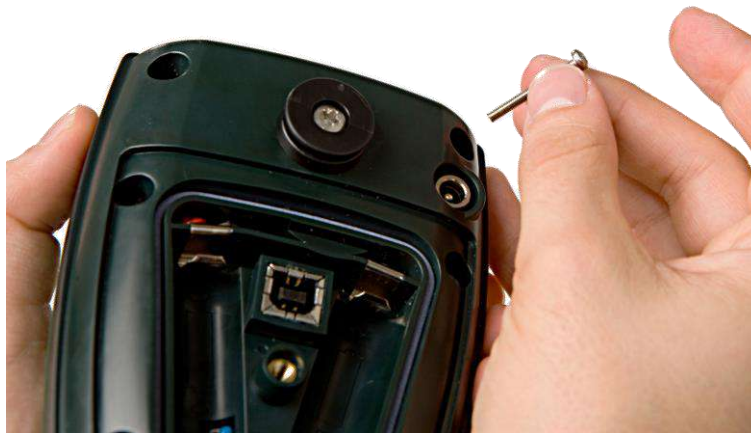
Figure 33 Replace the sensor cap and secure the screws
