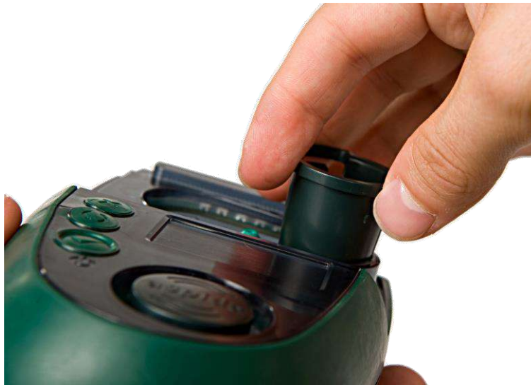
Figure 31 Remove the extraction tool
