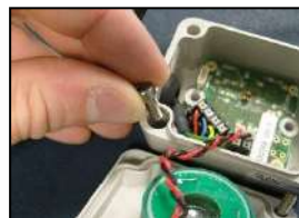
2) Insert the supplied M4 cap screws into each mounting hole
