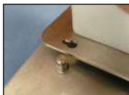
8) Align mounting hole with standoff
