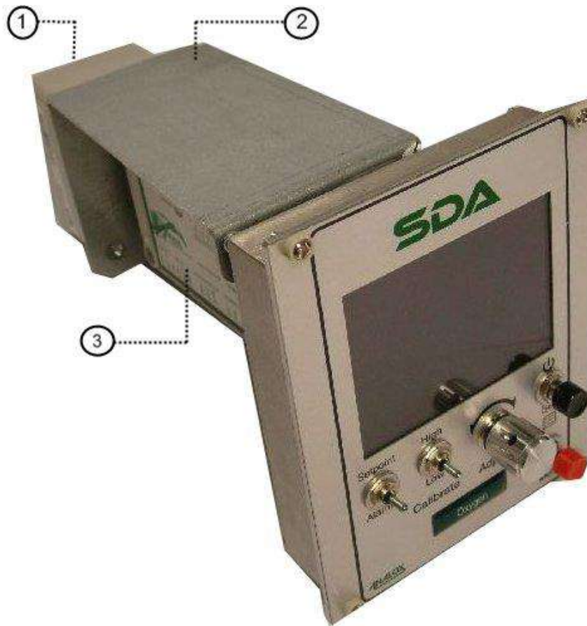
Figure 23 Assembly with the combined mounting bracket
