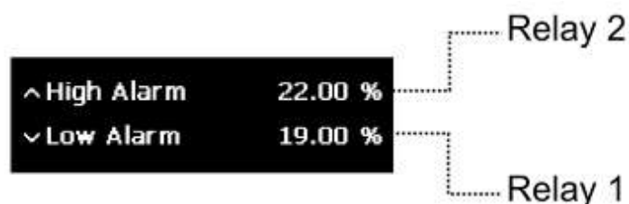
Figure 47 Alarm relay mapping
