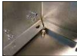
2) Align mounting hole with standoff
