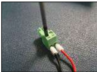
4) Secure using a terminal driver
