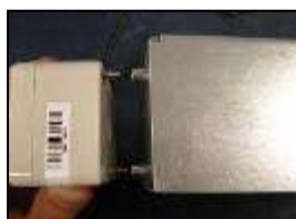
4) Align M4 cap Screws with standoffs
