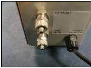
1) Remove bulkhead pipe securing nuts
