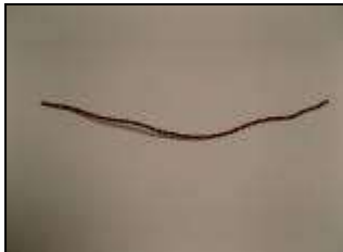
Cut a suitable length of 7/0.2mm red/black twisted wire
