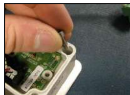
2) Insert the supplied M4 cap screws into each mounting hole
