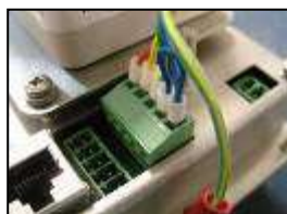
10) Connect MEC sensor
