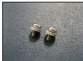
7) Remove 2 x M3 x 6mm Pozi Pan Screws and Nordlock washers from rear of monitor
