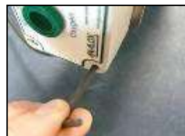
5) Tighten the M4 cap Screws with a 3mm hex key
