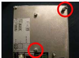
7) Remove 2 x M3 x 6mm Pozi Pan Screws and Nordlock washers from rear of monitor
