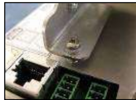
3) Secure in place with the 2 x M3 x 6mm Pozi Pan Screws and Nordlock washers from rear of monitor
