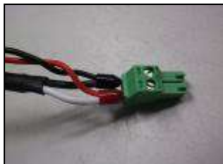
Connect the linked end to the remaining two way connector as shown
