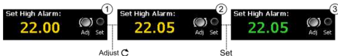
Figure 37 Example of alarm set-point adjustment
