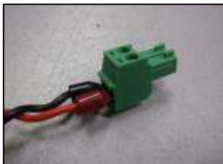
Crimp the free end of the red/black twisted wires with red and black 1.5mm bootlace ferrules and connect to the two way connector supplied with the SDA
