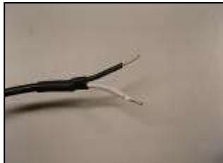
Remove the 2 way connector and bootlace ferrules from the cable and strip back 7mm
