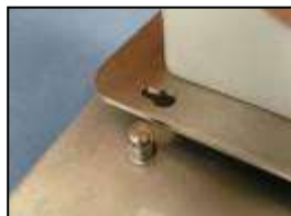
8) Align mounting hole with standoff
