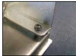
3) Secure in place with the 2 x M3 x 6mm Pozi Pan Screws and Nordlock washers from rear of monitor
