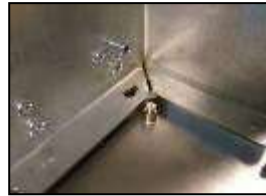
2) Align mounting hole with standoff
