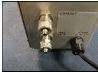
1) Remove bulkhead pipe securing nuts
