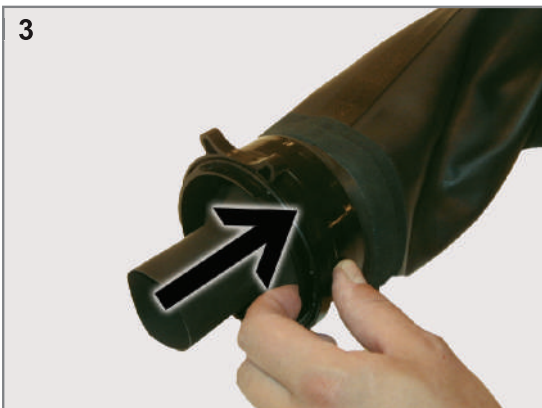
3. Align the thumb grips with the rubber tape of the sleeve to simplify donning. Press the lock ring into the male bayonet ring from inside the sleeve. Press until it fits to the inner edge of the male bayonet ring.
