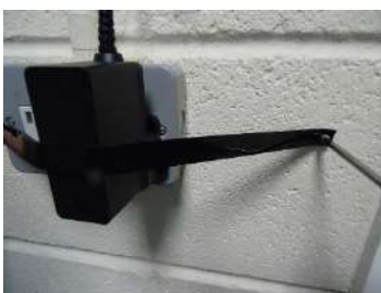
The plug-in PSU is supplied with a securing strip, wall plugs and screws to reduce risk of accidental disconnection or tampering
