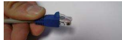
Slide boot back over lock clip
