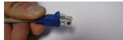
Slide boot back over lock clip
