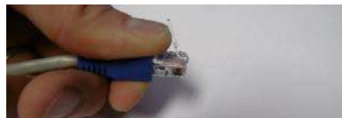
Pull boot back to access lock clip
