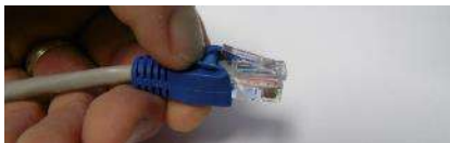
Pull boot back to access lock clip
