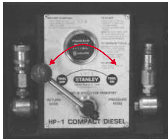
Figure 4. Control Panel to "ON" Position
