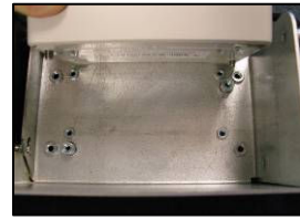
3) Align screws with standoffs
