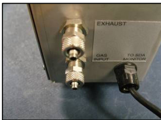
1) Remove bulkhead pipe securing nuts
