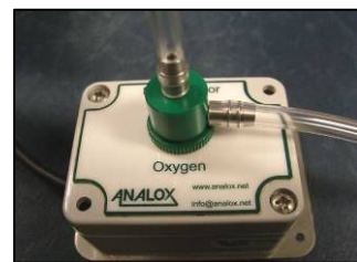
2) Connect flow adaptor to the inlet of the MEC O2 sensor
