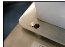
8) Align mounting hole with standoff
