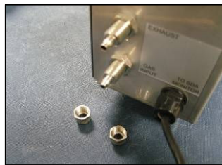
1) Remove bulkhead pipe securing nuts
