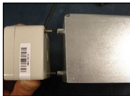
4) Align M4 cap Screws with standoffs
