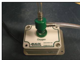
2) Connect flow adaptor to the inlet of the MEC O2 sensor
