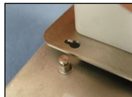
8) Align mounting hole with standoff
