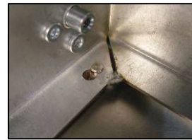
2) Align mounting hole with standoff
