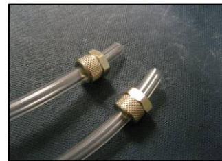
2) Fit securing nuts to pipes
