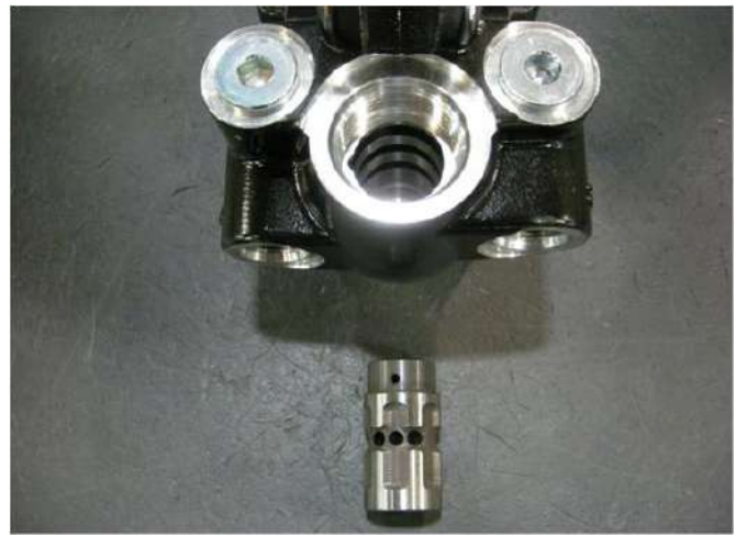
New Style – Uses no sleeve in spool bore.
