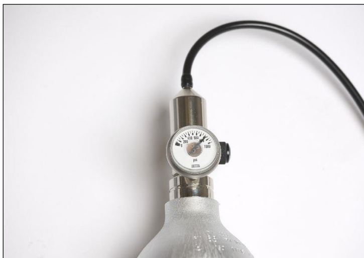
Figure 26 Flow Regulator Fitted to Calibration Bottle
