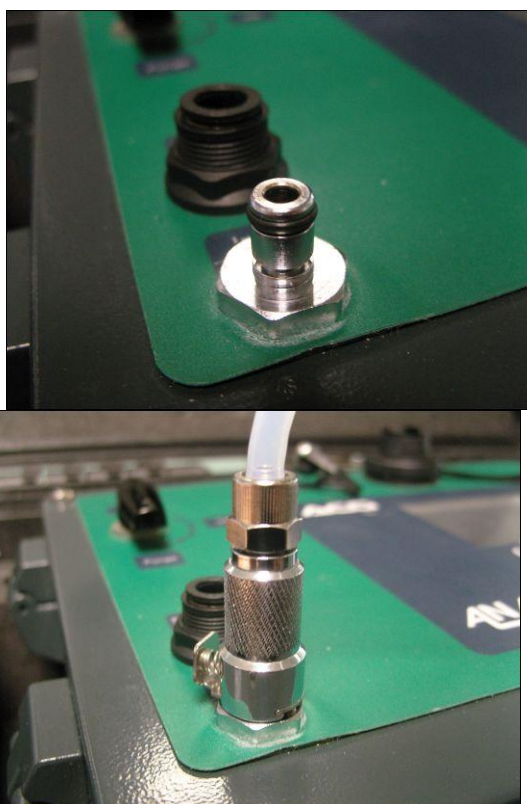
Figure 27 Connecting Calibration Fitting to ACG+ Calibration Port
