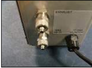
1) Remove bulkhead pipe securing nuts
