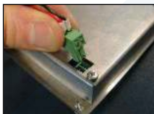
5) Connect to the DC input on the rear of the monitor
