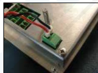
5) Connect to the DC input on the rear of the monitor
