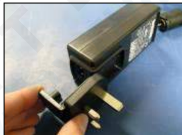
Select the correct plug type and insert into PSU as shown
