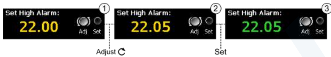
Figure 38 - Example of alarm set-point adjustment
