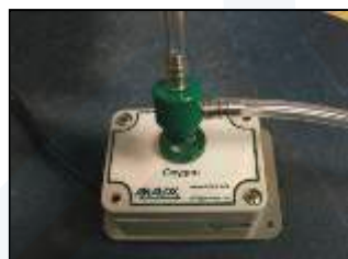
2) Connect flow adaptor to the inlet of the MEC sensor
