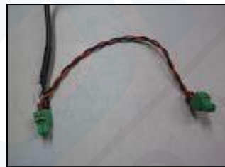
The PSU is now ready and can be connected to two SDA monitors as described in section 2.2.2 step 5
