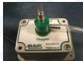
2) Connect flow adaptor to the inlet of the MEC sensor
