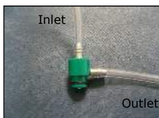
1) Connect pipe work to flow adaptor
