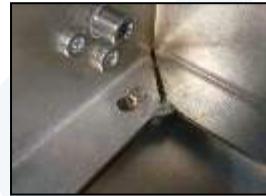
2) Align mounting hole with standoff
