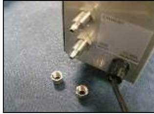
1) Remove bulkhead pipe securing nuts
