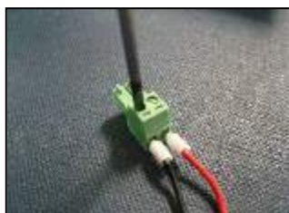
4) Secure using a terminal driver
