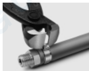
To release clamp, position the pincers across the ear and cut through
