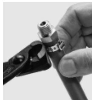
To release stepless clamps, grip end of band with pincers and pull off.
