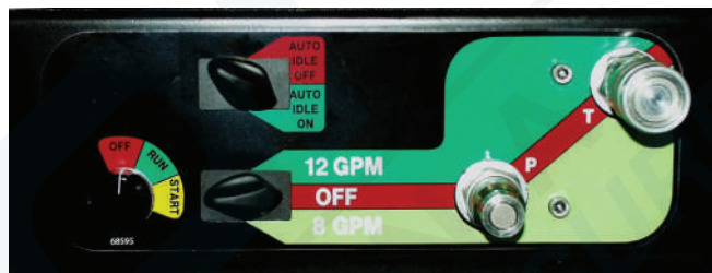
Figure 1. Panel Control Valve
