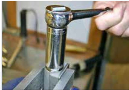
Step 5: Tighten the manifold plug (43) with a 7/8" socket to 90 in. lbs (10 Nm).
