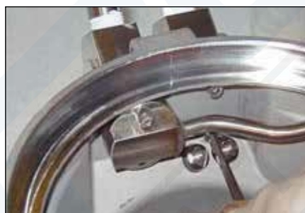
Step 36: Tighten short hex screw (39) onto the top of helmet using a 3/16" hex key to 80 in.lbs (9 Nm).
