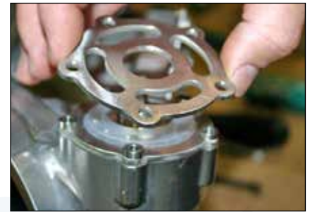
Step 25: Place exhaust valve cover (19) on top of spacer rings (17).
