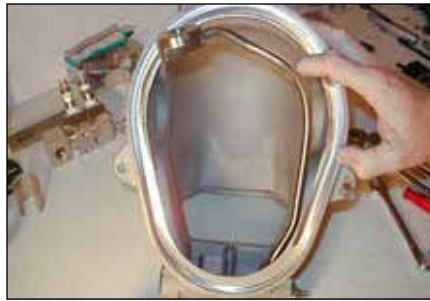
Step 9: Stick open end of airway assembly into swagelock connector (31).
