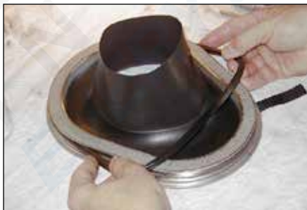
Step 1: Lightly lubricate quad ring (65) and install in groove of upper neck ring (66).
