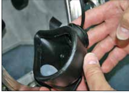
Step 8: Point microphone wire downwards.
