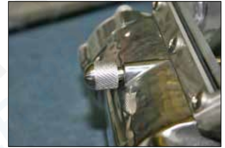
Step 12: Always check before diving to ensure that no threads are visible in order to prevent loosening the knob (64).
