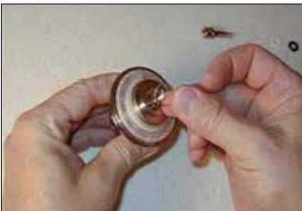
Step 11: Place two copper washers (56) on top of the valve seat (55) in the valve body (52).
