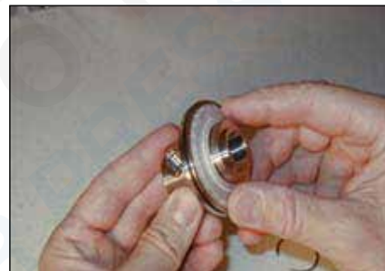
Step 6: Flapper exhaust valve (18) installed on valve body (52).
