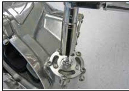
Step 17: Tighten the valve bonnet (60) with a 11/16" socket to 35 ft.lbs (47 Nm).
