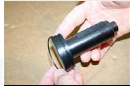
Step 8: Lubricate and install o-ring on outside of free flow plug. Place hook and loop strip on barrel.
