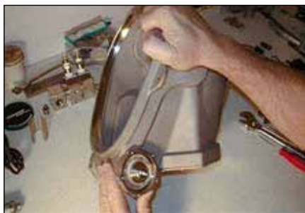
Step 2: Free flow / water dump valve in place.
