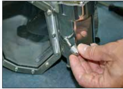
Step 11: Secure NCD knob (64) on the NCD shaft (62). Ensure that it is snug.
