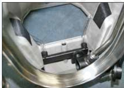
Step 5: Slide upper unit over the bracket of the lower unit.
