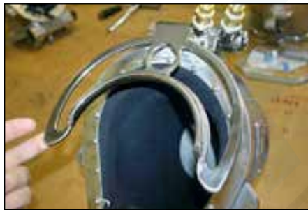
Step 1: Place front portion of neck dam into the front of the helmet. Use neck retainer (21) to push the back side of the neck dam in place.
