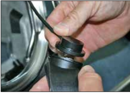
Step 7: Install microphone (30) in the right pocket of the oral-nasal mask (37).
