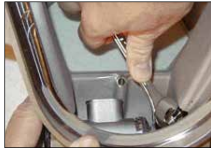
Step 7: Tighten swagelock connector (31) into free flow / water dump valve body (52) using 5/8" open end wrench to 45 in.lbs (5 Nm).
