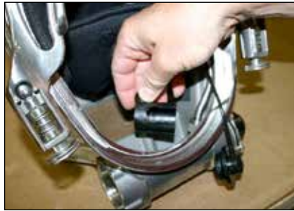
Step 7: Remove free flow barrel (32).
