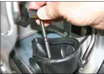
Step 10: Install nose clearing device (62) into the helmet shell (1).
