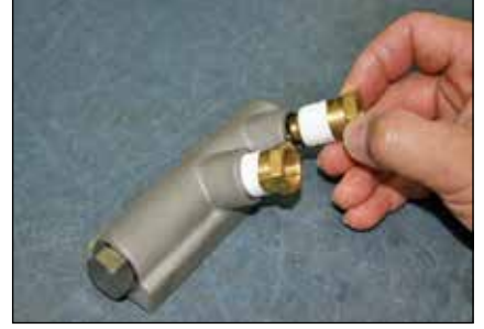
Step 9: Screw check valve (47) (with Teflon tape) into the 2nd port of the manifold body (45).
