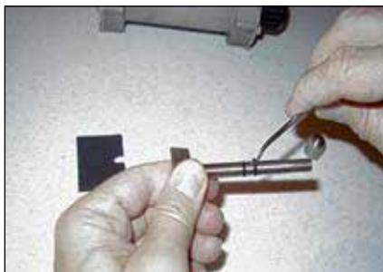
Step 2: Install two o-rings (63) into the grooves on the NCD shaft (62) using o-ring pick.
