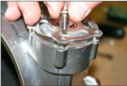
Step 26: Insert retainer port screws (11) and tighten by hand.
