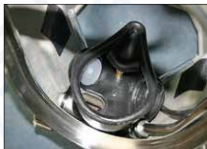
Step 13: Inside view of installed oral-nasal mask assembly.
