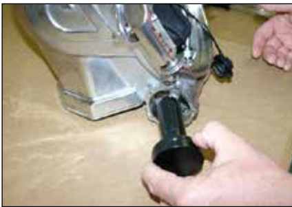
Step 9: Install free flow plug in helmet shell (1). Ensure hook and loop strip is facing inward.
