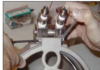
Step 40: Use a 3/16" hex key to hold the bolt (23) and 7/16" nut driver to hold the nut (22). Tighten until the nut touches the hinge. Adjust as required.
