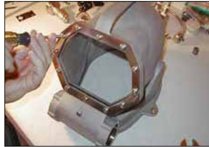
Step 9: Tighten all screws (11) to 45 in.lbs (5 Nm) with a Phillips #3 screwdriver.
