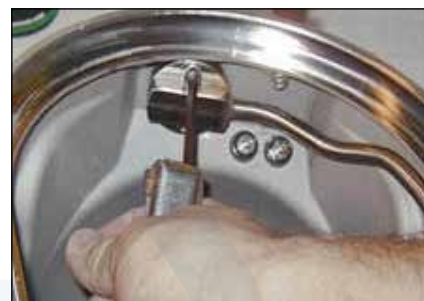
Step 34: Tighten the longer manifold hex screws (10) onto inner airway bracket using a 3/16" hex key to 80 in.lbs (9 Nm).
