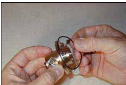
Step 4: Install o-ring (53) onto the valve body (52) groove.
