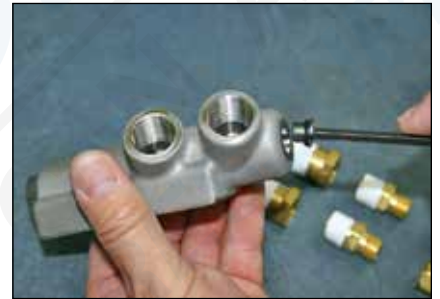
Step 6: Install o-ring (33) onto port plug (46). Using a 3/16" hex key, screw the port plug to the manifold body (45).
