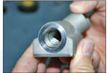
Step 3: Line up screen (44) with the end of threads in the manifold body (45).
