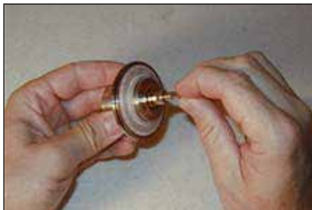
Step 10: Thread in the valve seat (55) with valve stem (57).
