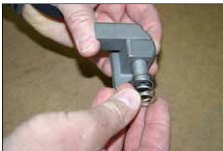
Step 4: Fit latch spring (8) over shaft of left latch (2) or right latch (3).
