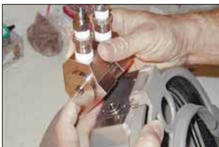
Step 32: Line up assembled manifold body (45) with the manifold insert (40) and holes.
