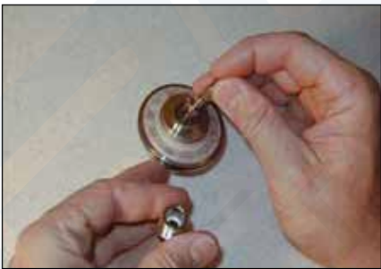
Step 14: Place the valve stem (57) into the valve body (52) over the seat (55).
