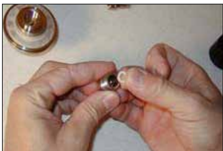
Step 13: Place Teflon washer (58) over the o-ring (59) in the valve bonnet (60).
