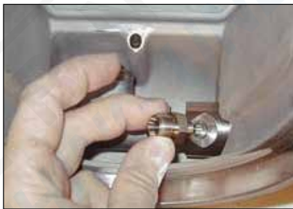
Step 6: Screw connector into free flow / water dump valve body (52).
