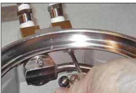
Step 35: Tighten short hex screw (39) onto the bottom of helmet using a 3/16" hex key to 80 in.lbs (9 Nm).
