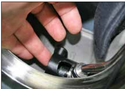
Step 2: Insert lower unit over the free flow / water dump valve body.
