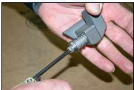
Step 7: Tighten manifold hex screw (10) using a 3/16" hex key to 80 in.lbs (9 Nm).
