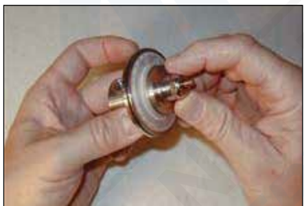
Step 16: Thread the valve bonnet (60) into the valve body (52).
