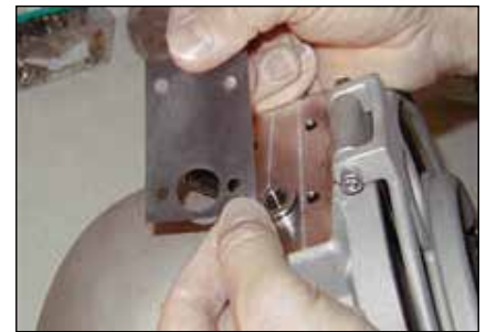
Step 31: Place the manifold gasket (42) over the back side of helmet shell (1) and line up the holes.
