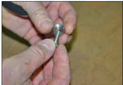
Step 5: Fit latch spring washer (9) onto manifold hex screw (10).
