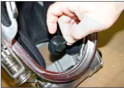
Step 12: Place hook and loop tab on base of microphone (30).
