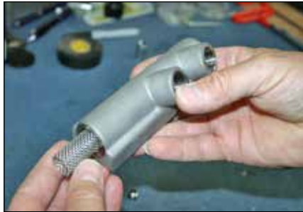
Step 2: Insert screen (44) into the manifold body (45). Failure to install may cause debris to block the flow of gas to the diver.
