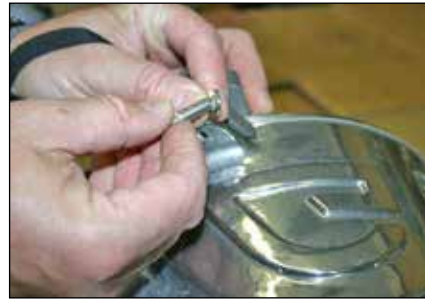
Step 9: Fit latch spring washer (5) onto latch screw (4).
