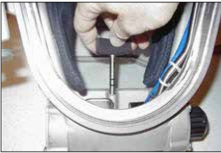
Step 41: Install nose clearing device (62) through the inside of helmet shell (1).
