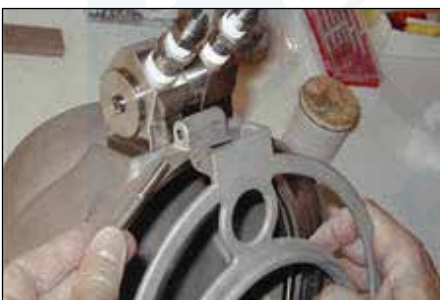
Step 38: Line up neck retainer (21) with the hinge and insert the neck retainer bolt (23).
