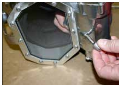
Step 15: Place NCD knob (64) on NCD (62) to secure in place.
