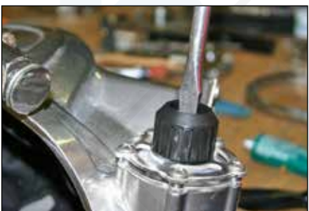
Step 29: Tighten nut (20c) until snug using a 3/8" flat blade screwdriver.
