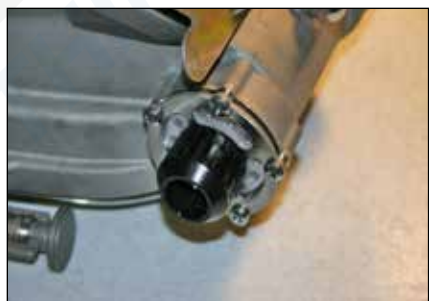
Step 30: Double water dump exhaust installed.
