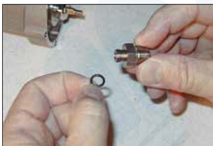
Step 5: Place o-ring (33) on swagelock connector (31).
