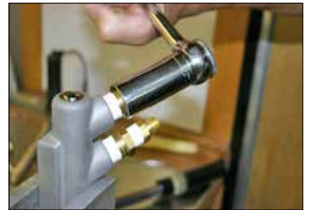
Step 12: Tighten both check valve assemblies to the manifold body (45) with an 7/8" socket. Replace caps (50).
