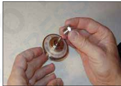
Step 15: Place the valve bonnet assembly over the valve stem (57) into the valve body (52).
