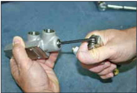
Step 7: Tighten port plug (46) with a 3/16" hex key until to 45 in. lbs (5 Nm).
