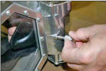
Step 1: Remove nose clearing device (NCD) knob (64).
