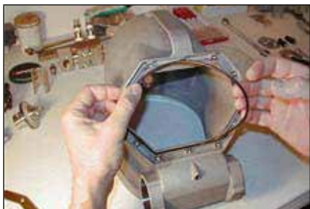
Step 1: Place o-ring (14) in the port groove.
