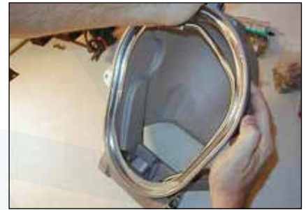
Step 10: Press airway assembly (29) inside the helmet shell (1).
