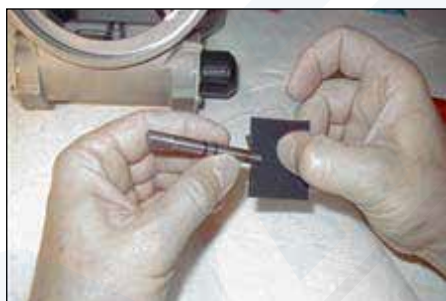
Step 4: Place neoprene nose pad (61) over nose cleaning device (62) as shown.
