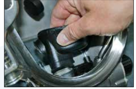
Step 9: Install oral-nasal mask (37) onto the regulator mouthpiece.
