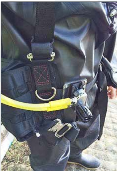
Lower hose routed from bailout cylinder, upper hose routed to helmet
