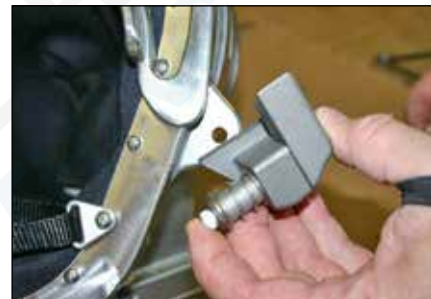
Step 8: Fit assembled latch base left (6) or latch base right (7) onto correct side of helmet shell (1).
