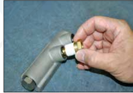
Step 8: Screw check valve (47) (with Teflon tape) into the first port of the manifold body (45).
