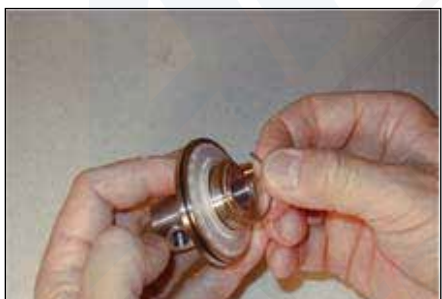
Step 7: Install snap ring (54) in the groove on the valve body (52).
