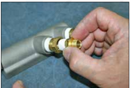
Step 10: Screw scuba fitting (48) (with Teflon tape) to the first check valve (47) and tighten firmly.
