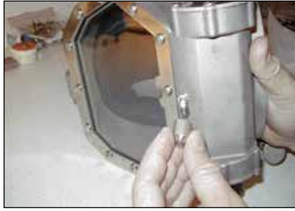
Step 42: Screw NCD knob (64) into the nose clearing device (62).
