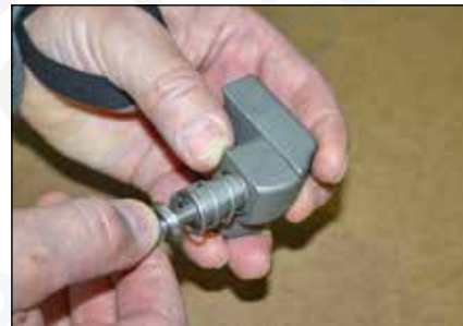
Step 6: Insert manifold hex screw (10) and washer (9) into shaft of left latch (2) or right latch (3).
