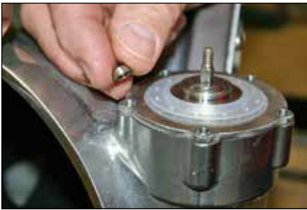
Step 23: Place all spacer rings (17) onto the dual exhaust seat (16).
