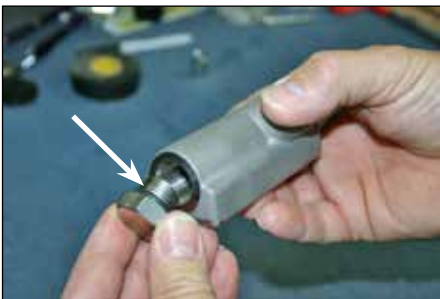
Step 4: Install o-ring (26) onto manifold plug (43). Screw manifold plug to the manifold body (45).
