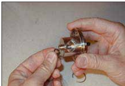
Step 2: Install small o-ring (51) onto valve body (52).
