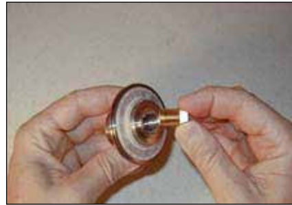
Step 9: Place valve seat (55) into the valve body (52).
