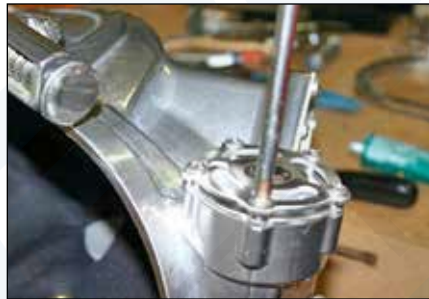
Step 27: Tighten screws (11) using a Phillips #3 screwdriver to 45 in.lbs (5 Nm).
