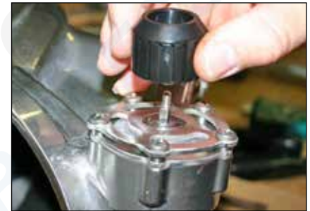
Step 28: Place handwheel knob (20a), spring (20b) and nut (20c) onto the free flow / water dump valve stem (57).
