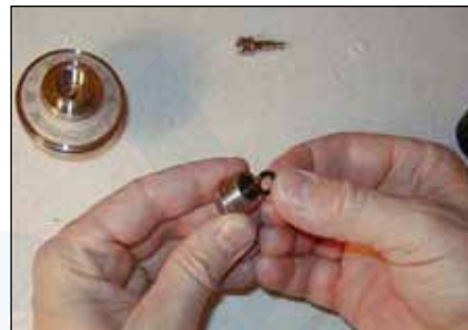
Step 12: Place o-ring (59) into the valve bonnet (60).
