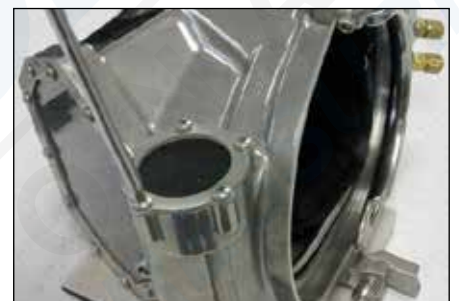
Step 11: Tighten exhaust valve cover screws using a Phillips #3 screwdriver to 45 in.lbs (5 Nm).
