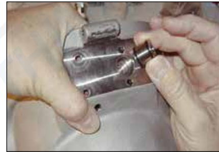
Step 15: Place manifold insert (40) through the wall of the helmet shell (1) into the airway bracket socket.
