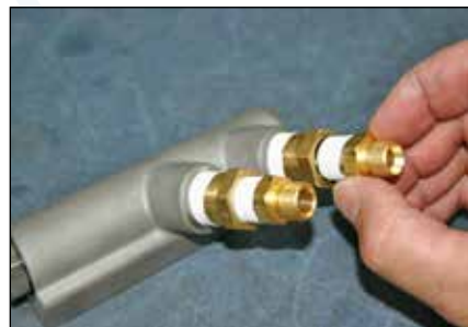
Step 11: Screw hose fitting (49) (with Teflon tape) to the 2nd check valve (47) and tighten firmly.
