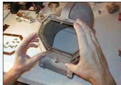
Step 3: Place face port (13) into the helmet shell (1).
