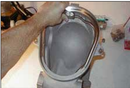
Step 11: Press bracket end of the airway assembly (29) to the back wall of the helmet shell (1).
