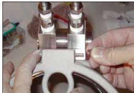
Step 39: Put the neck retainer nut (22) on the neck retainer bolt (23).
