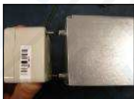
4) Align M4 cap Screws with standoffs
