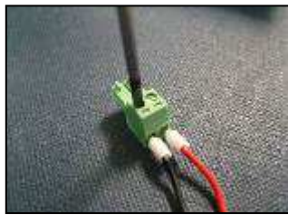
4) Secure using a terminal driver
