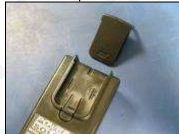
Press clip and remove blanking cover
