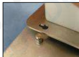
8) Align mounting hole with standoff
