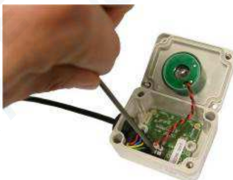
Figure 47 - Disconnecting the cell
