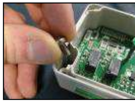
2) Insert the supplied M4 x 8mm Pozi-Pan Screws into each mounting hole
