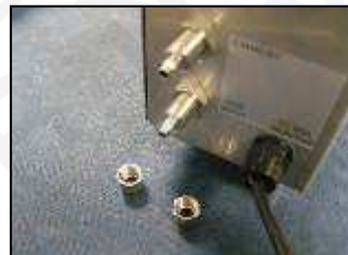
1) Remove bulkhead pipe securing nuts
