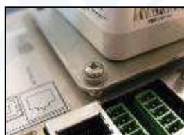
9) Secure bracket with 2 x M3 x 6mm Pozi-Pan Screws and Nordlock washers
