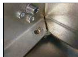
2) Align mounting hole with standoff
