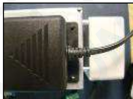
1) Align the PSU mounting holes with the four outer M4 threaded inserts on the bracket
