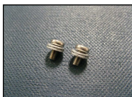
1) Remove 2 x M3 x 6mm Pozi Pan Screws and Nordlock washers from rear of monitor
