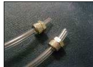
2) Fit securing nuts to pipes
