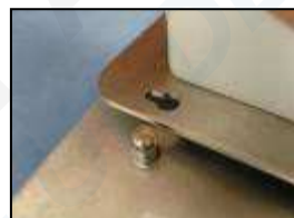
8) Align mounting hole with standoff
