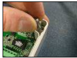
2) Insert the supplied M4 x 8mm Pozi-Pan Screws into each mounting hole
