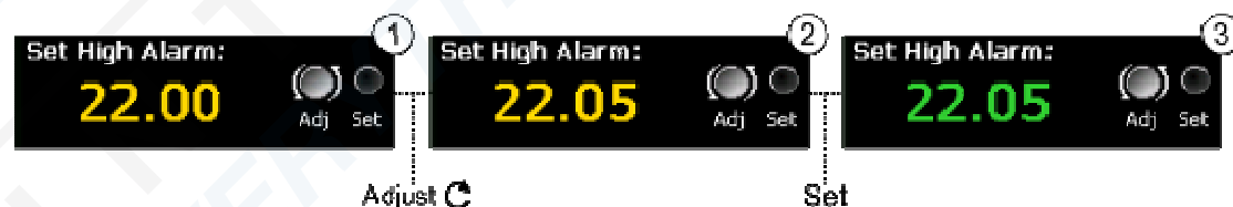
Figure 31 - Example of alarm set-point adjustment
