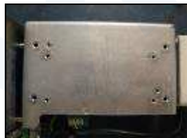
1) Align the PSU mounting holes with the four outer M4 threaded inserts on the bracket
