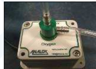
2) Connect flow adaptor to the inlet of the MEC sensor
