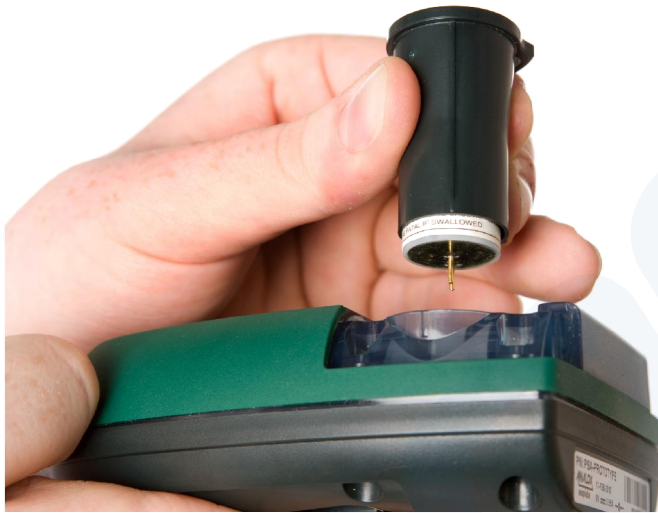
Figure 25 - Align the new sensor with the Aspida device
