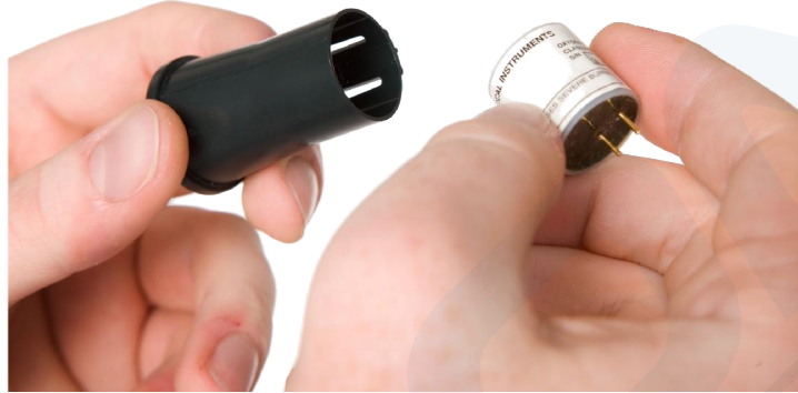
Figure 23 - Insert the new sensor into the extraction tool
