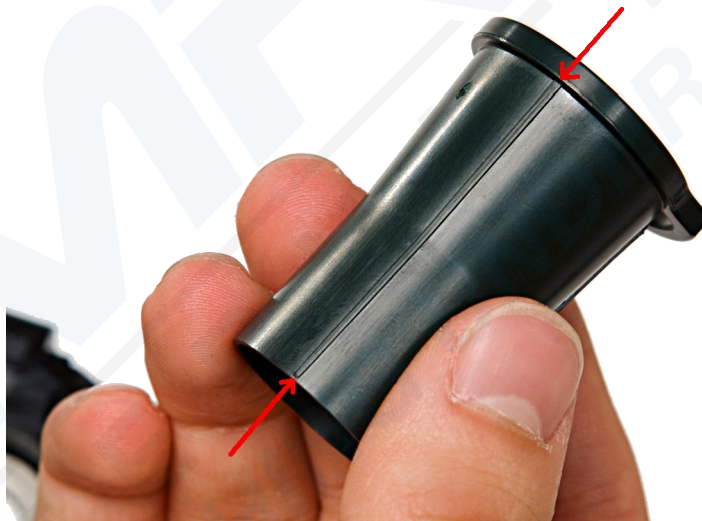
Figure 18 - Locate the alignment rib
