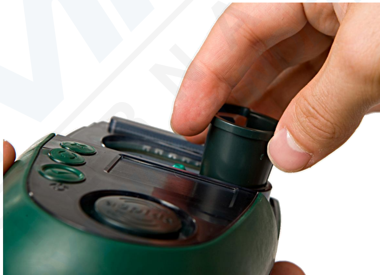
Figure 26 - Remove the extraction tool
