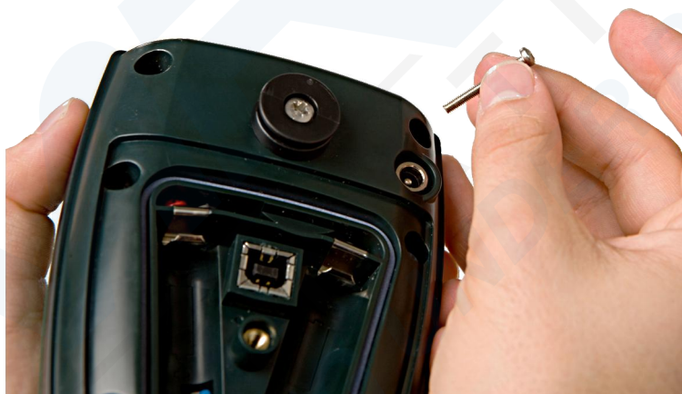
Figure 28 - Replace the sensor cap and secure the screws
