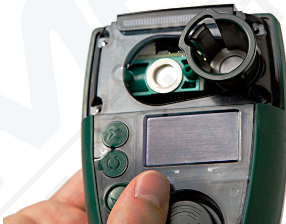
Figure 20 - Correct extraction tool position
