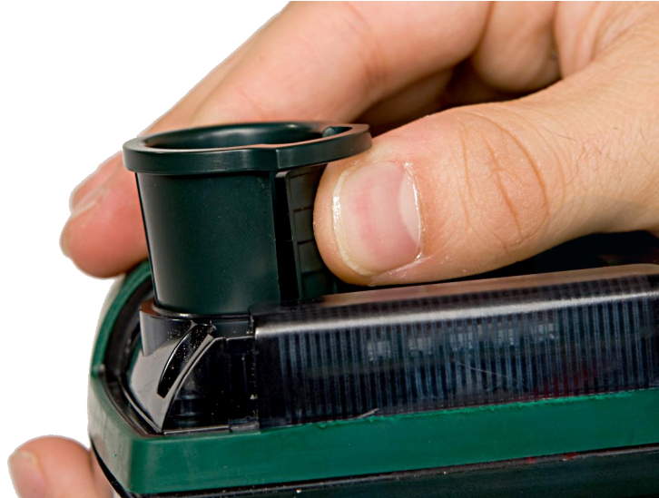
Figure 21 - Squeeze the extraction tool
