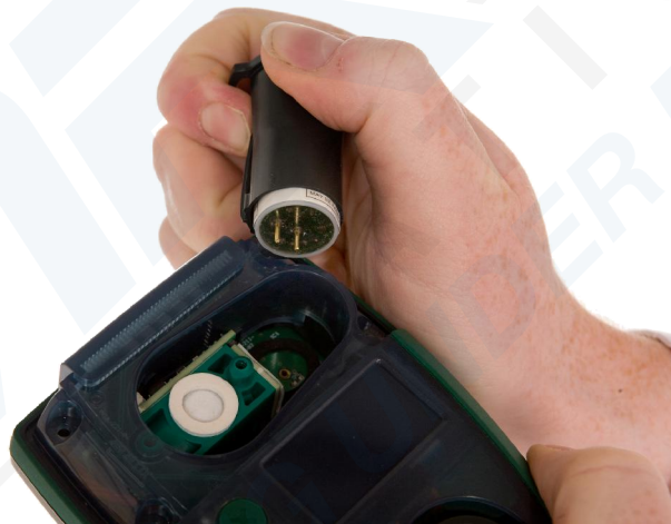
Figure 22 - Removing the oxygen sensor
