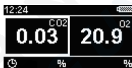
Figure 7 - The main gas display showing that to user has exceeded their TWA exposure to carbon dioxide
