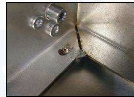
2) Align mounting hole with standoff
