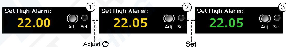
Figure 24 - Example of alarm set-point adjustment
