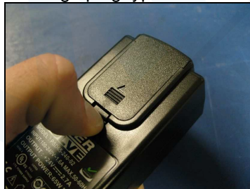
Press clip and remove blanking cover
