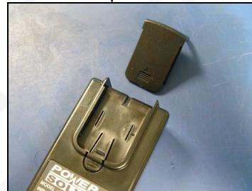
Press clip and remove blanking cover
