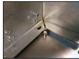
2) Align mounting hole with standoff
