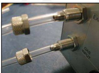
3) Fit Gas Input and Exhaust pipe-work to bulkheads
