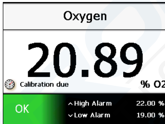
Figure 26 - A calibration adjustment reminder
