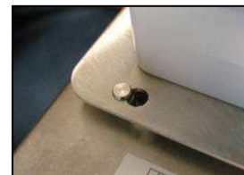
8) Align mounting hole with standoff
