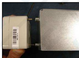
4) Align M4 cap Screws with standoffs
