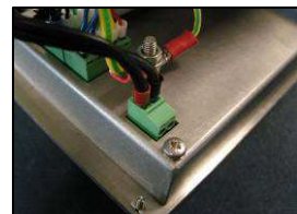
3) Connect to the DC input on the rear of the monitor
