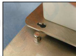
8) Align mounting hole with standoff
