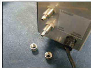
1) Remove bulkhead pipe securing nuts
