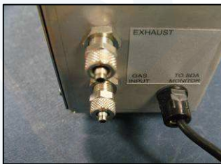
1) Remove bulkhead pipe securing nuts
