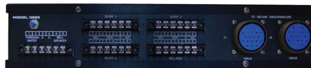
3222 BELL ROUTING PANEL REAR CONNECTIONS
