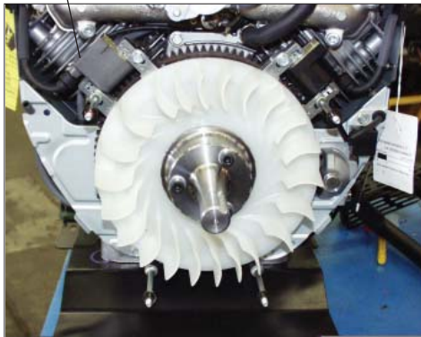
Fan Cover Removed From Honda Engine
