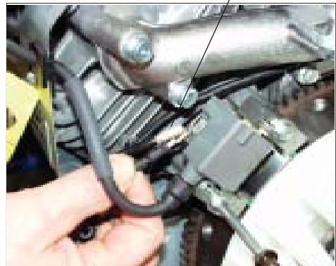
Receptacle with 1/4-inch Double Tab Connected to Pick-up Coil
